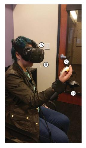
**Figure 1.** A participant in the touch and scent present condition. The figure depicts: (A) an HTC Vive HMD, (B) a cotton bud dipped in chocolate donut scented aromatic oil to simulate the scent of a donut and attached to the HMD using Velcro strips, (C) a fake rubber donut to simulate the sense of touch, and (D) the HTC Vive hand controller.
